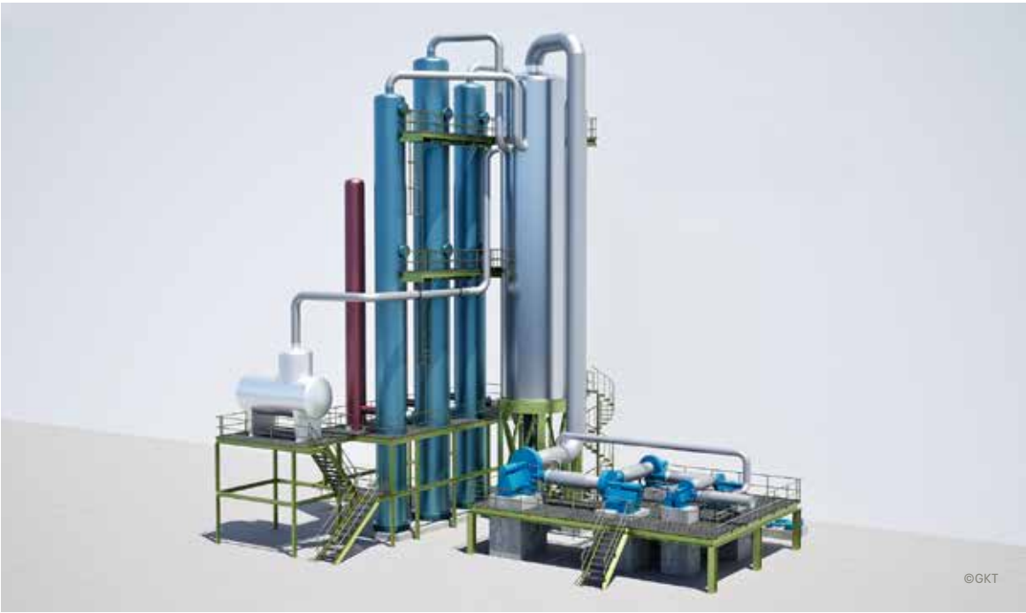
VarioVAP system – combining heat streams from different sources and media.
