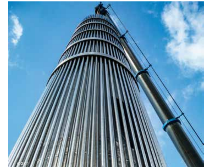
Short-path evaporator with integrated condenser
